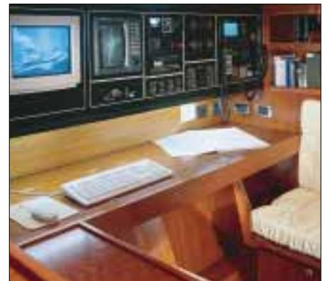
generated by Maxsea, a navigational program interfaced with the electronic instruments. Finally, all of the documentation and operation manuals for the boat are accessible on the 15" color liquid crystal screen.
