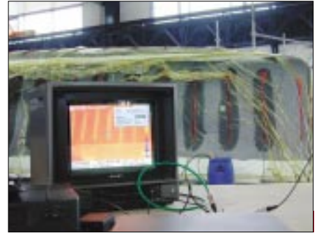
▼ 4 - Throughout the process, temperature is infra-red controlled.
