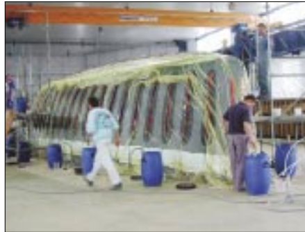
▲ 1 - Infusion starts as resin flows through the fabric, pumped in by the vacuum system.
