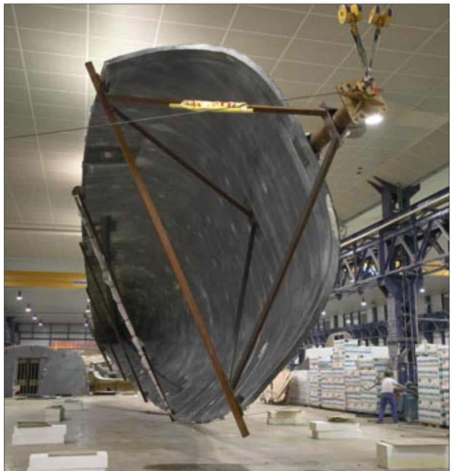
The final adjustments of the composite keel trunk and the stainless keel. The installation of the 30 ton bulb is completed when it is in place in the yacht.
