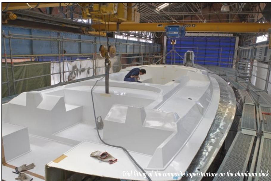
*Trial fitting of the composite superstructure on the aluminum deck*
