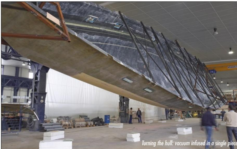
Turning the hull: vacuum infused in a single piece
